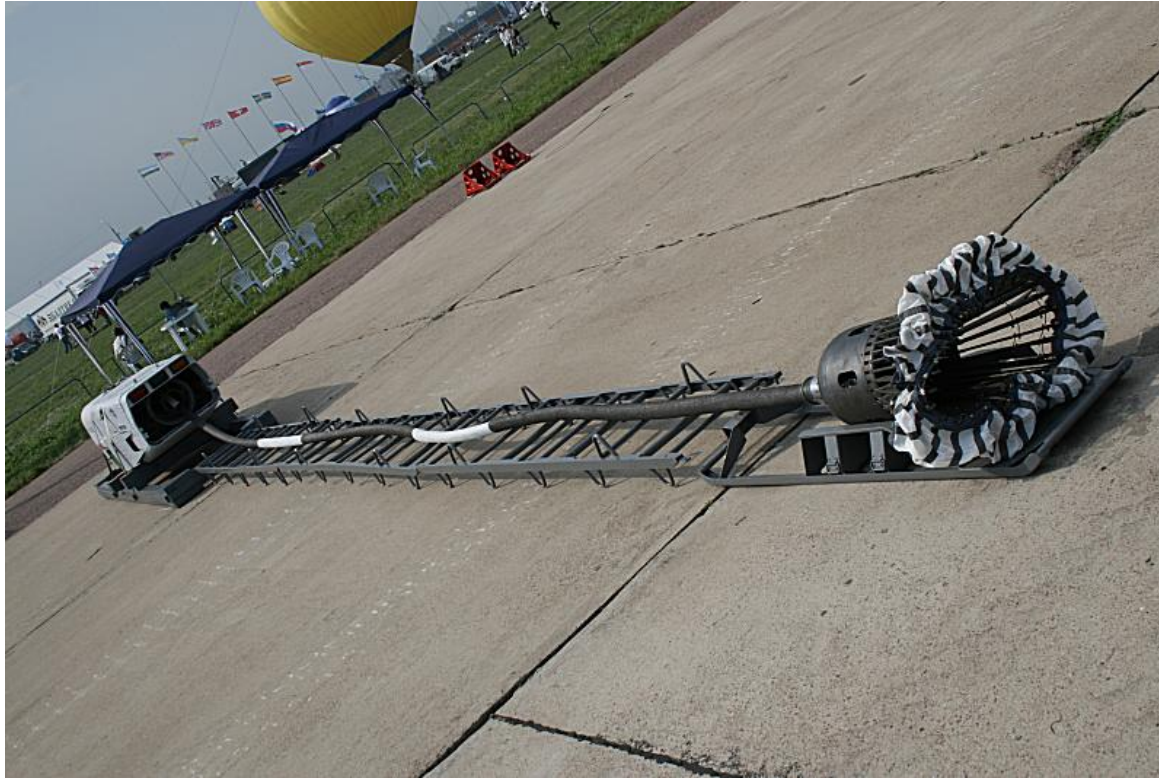
УПАЗ-1М Unit during maintenance procedures' performance
