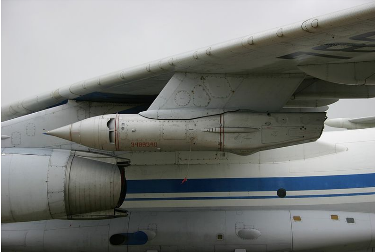
УПАЗ-1М Unit under the wing of Il-78 aircraft
